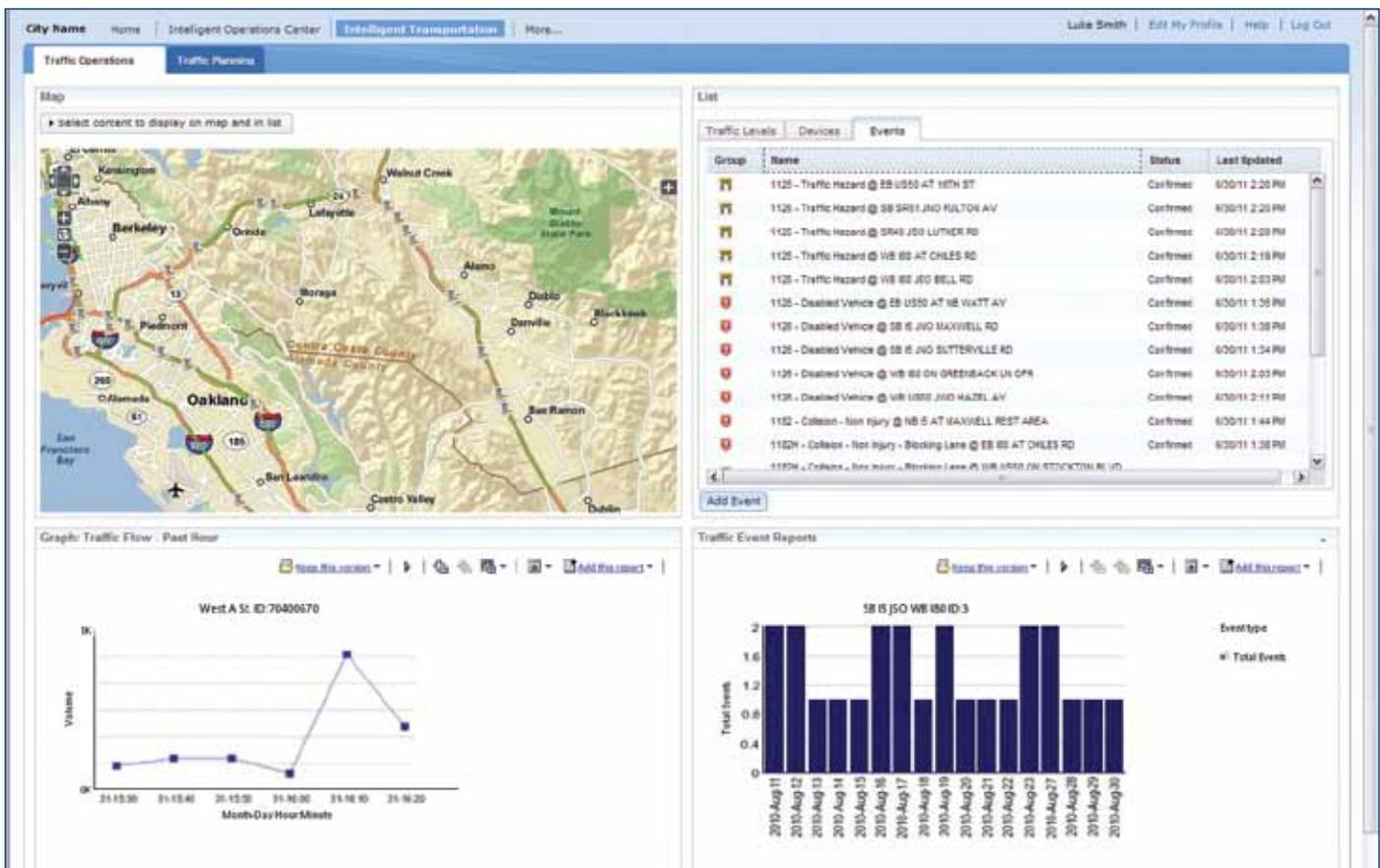
Figure 1: The Traffic Operations view is used to monitor and analyze the current traffic flow, events and performance of the traffic network. It provides a visual representation of current traffic data collected by sensors in the field of the geographical traffic region.
